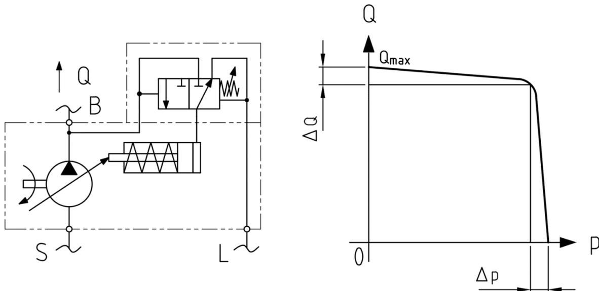
Fig. 2. Pump with pressure regulator
