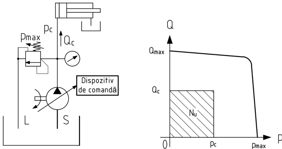
**Fig. 7.** Direct control of pumps with variable flow
