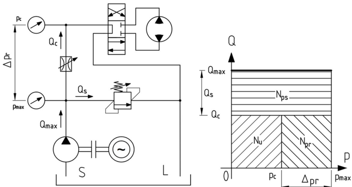
Fig. 1. Fixed displacement pump in "open centre" hydraulic system
