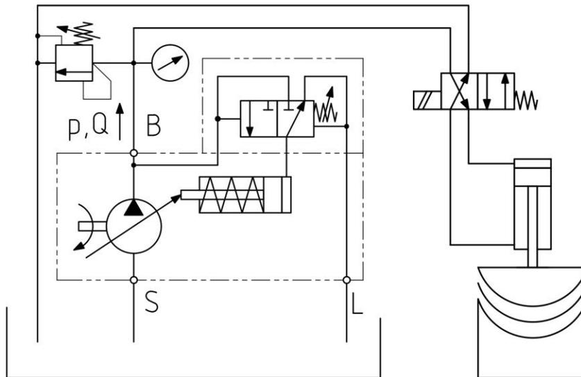
**Fig. 3.** Application of a pump with pressure regulator
