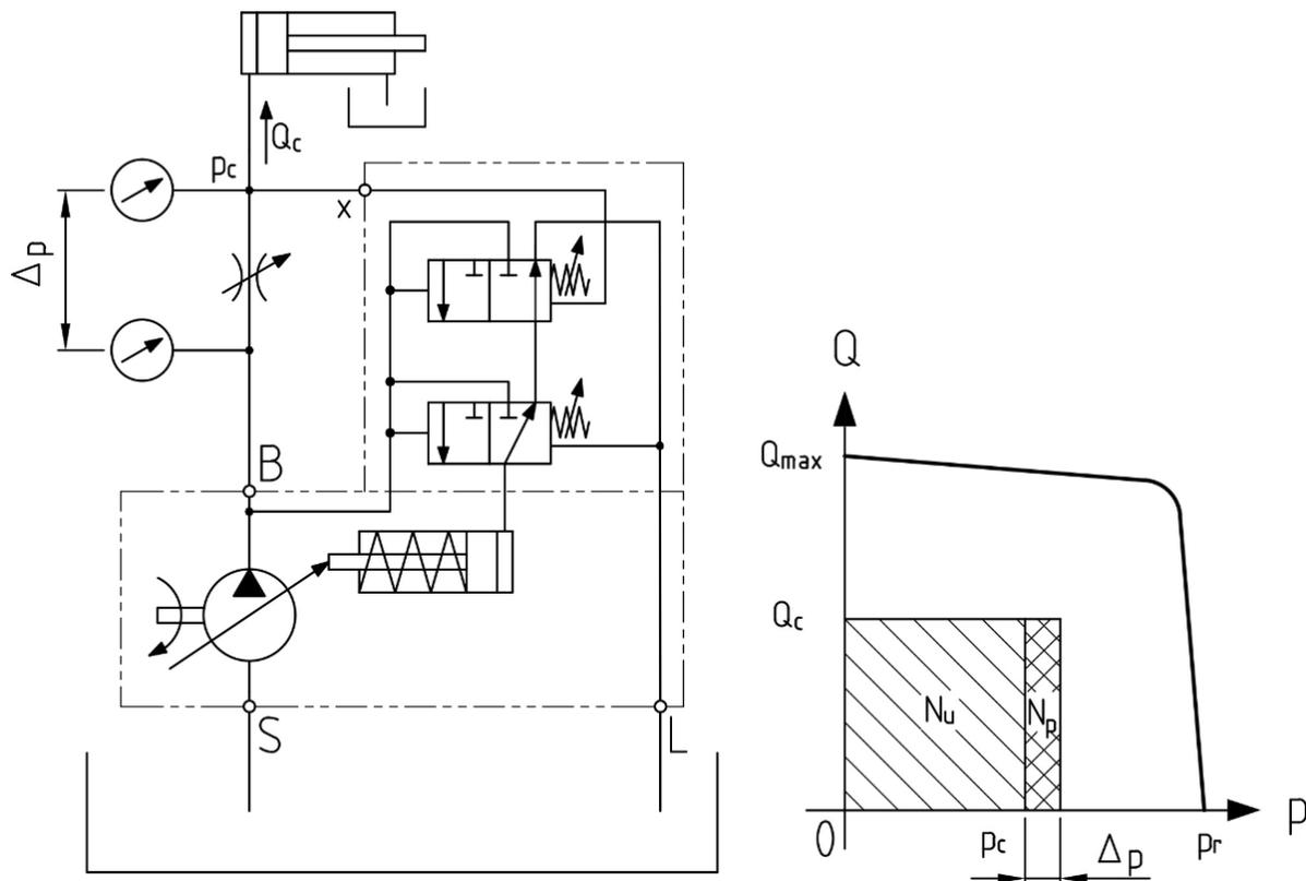
Fig. 5. Pump equipped with flow and pressure regulator
