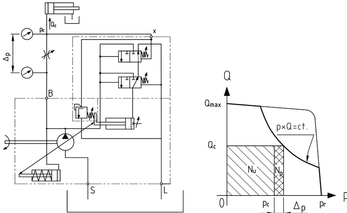
Fig. 6. Pump with pressure, flow and power regulator
