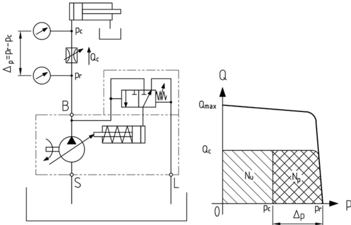
**Fig. 4.** Flow control in pumps equipped with pressure regulator
