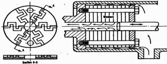
Fig. 5. Etched washer valve concept
