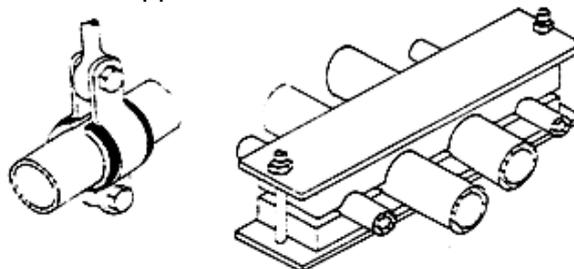
**Fig. 8.** Vibrating and isolating pipe clip and Pipe clamp block with vibrating isolating material
