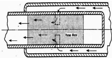
Fig. 4. Porous metal valve concept
