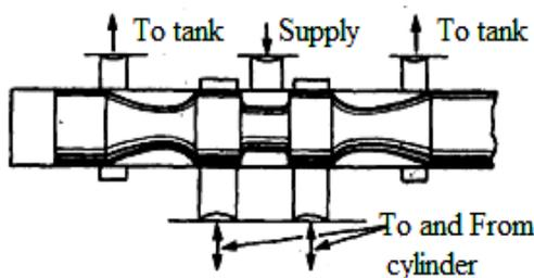
Fig. 6. DCV spool contoured for low noise
