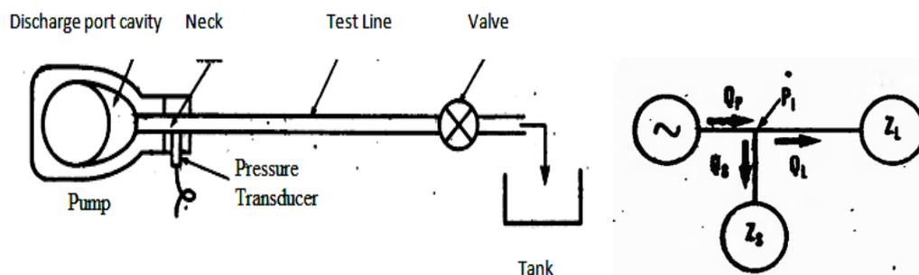
Fig. 2. Schematic diagram of pump circuit
