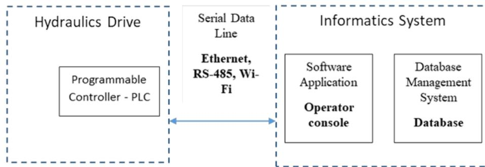
Fig. 1. Hardware architecture
