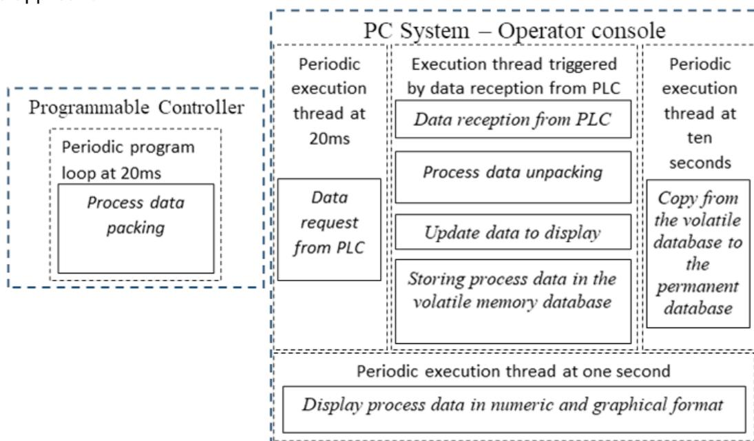
Fig. 2. Software architecture
